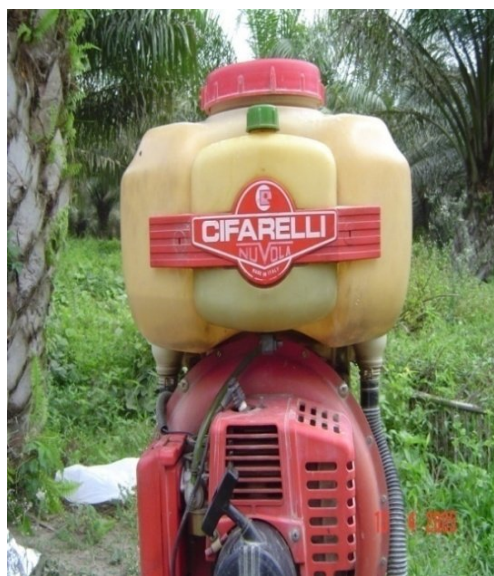
Figure 1. Powered sprayer machine used to apply insecticide on the experiment of spraying Vs. fogging application.
