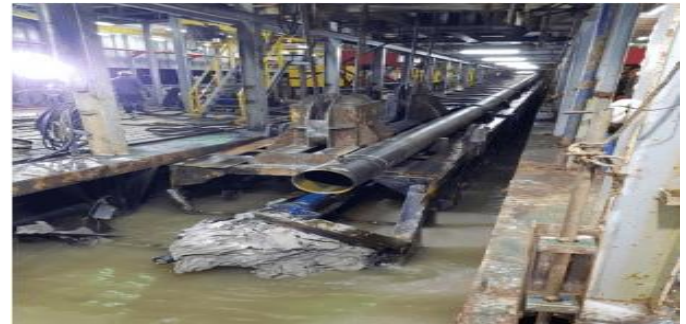
Gambar 4. Patah ladder KIP Timah 19
