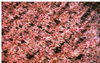
Fig. 3.29 Modified surface of aluminum foil by spark discharge
