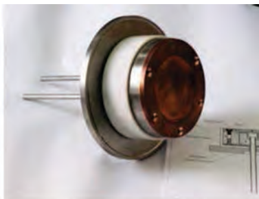
○ Fig. 4.4 Vacuum unit VUP-5M: a – photograph of the vacuum unit; b – photograph of the material-saving magnetron
