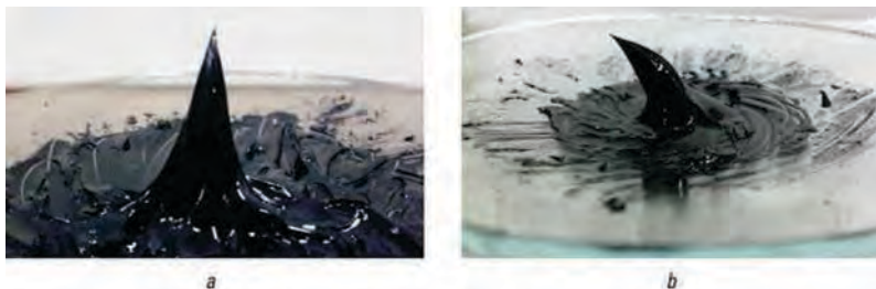
Fig. 3.7 Image of "standing paste": a – an example of the existing structure of the paste; b – deformation of the paste during a push
