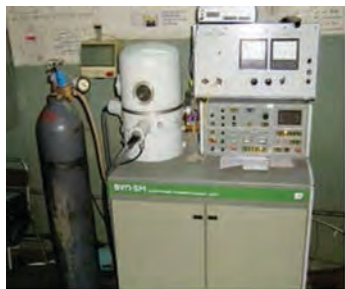
○ Fig. 4.4 Vacuum unit VUP-5M: a – photograph of the vacuum unit; b – photograph of the material-saving magnetron
