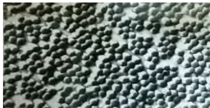
Fig. 3.31 Surface of ultrathin film of BM-12 acrylate suspension (x13000, electron microscopy)
