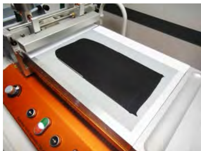
◉ Fig. 3.47 Image of the electrode on the device Dr. Blade after applying the YP-50F activated carbon suspension and the combination of Solef XPH-884 aqueous emulsion with NaCMC in a ratio of 2:1
