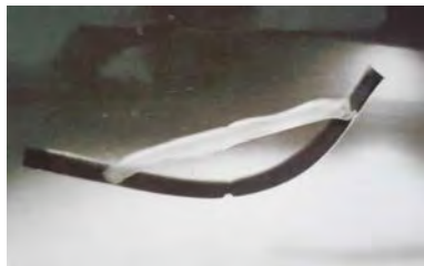
Fig. 3.21 Shrinkage of the polymer after drying
