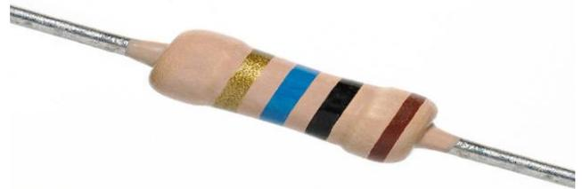
Gambar 2.5 Resistor karbon
