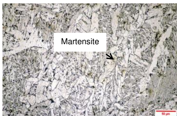
Figure 8. Microstructure at weld metal with WPS
