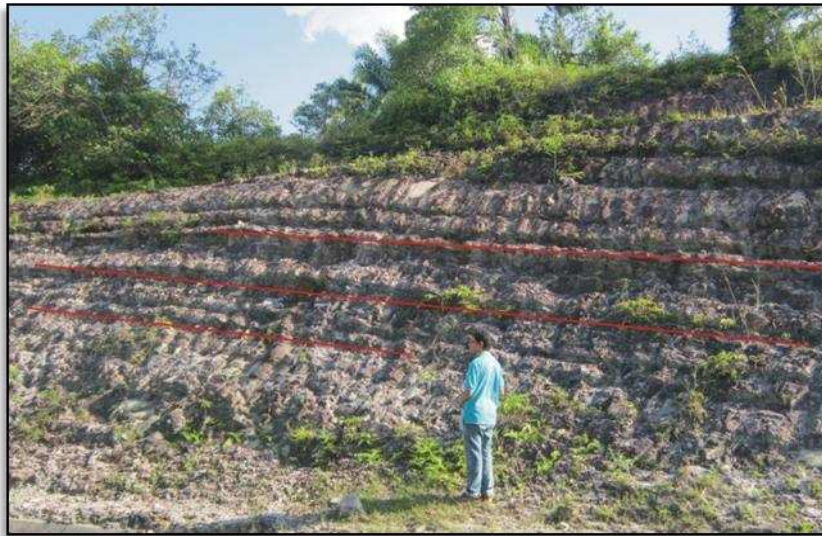
Figure 7. Photograph shows one parallel bedding planes in location 4 which is striking SE ( 107^\circ ) with gently dipping around 26^\circ towards southwest
