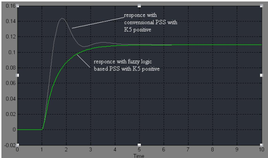
Figure 7. Comparison of angular position with conventional PSS (lead-lag) and fuzzy logic based PSS with K5 positive
