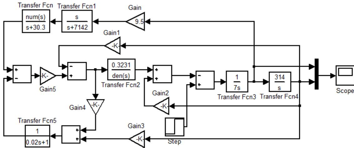
Figure 4. Simulink model with AVR and PSS
