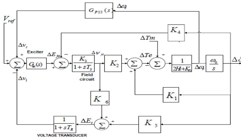
Figure 1. Block diagram representation with AVR and PSS
