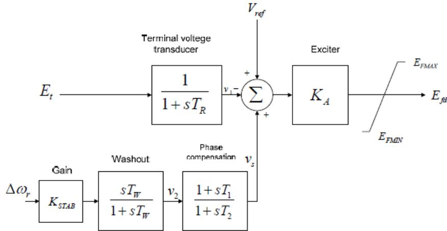
Figure 2. Thyristor excitation system with AVR and PSS
