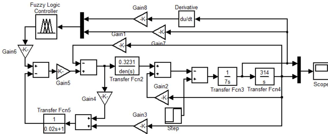
Figure 5. Simulink model with fuzzy logic based PSS
