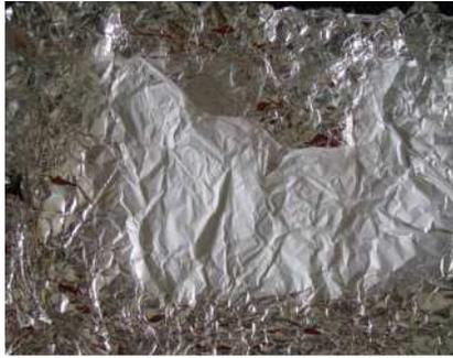
**Gambar 3. Serat nano PVA hasil percobaan awal electrospinning**
