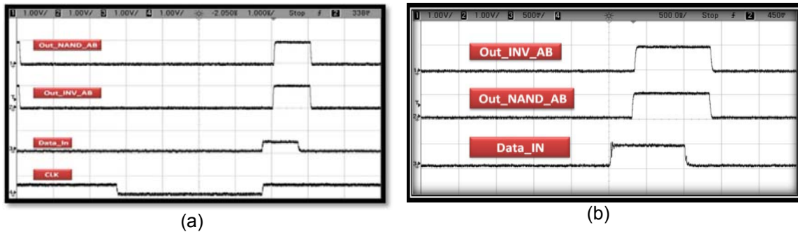
Figure 8. Measurement results of NAND AB and INV AB and chain at V_{DD} = 400 mV. (a) Dynamic mode. (b) Static mode.
