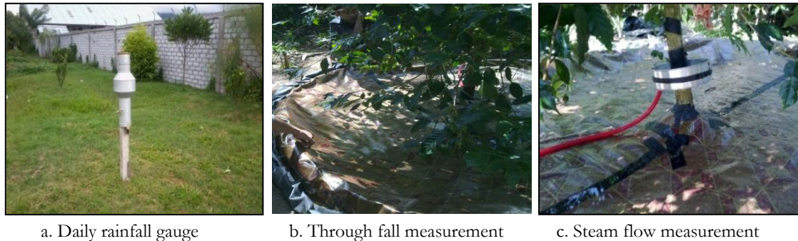
Figure 1. Instruments of rainfall interception loss measurement consist of daily rainfall gauges (a); daily through fall measurement (1b); and daily steam flow measurement (1c).
