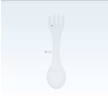
Gambar 10. Cacat weld line lokasi gate 3.
