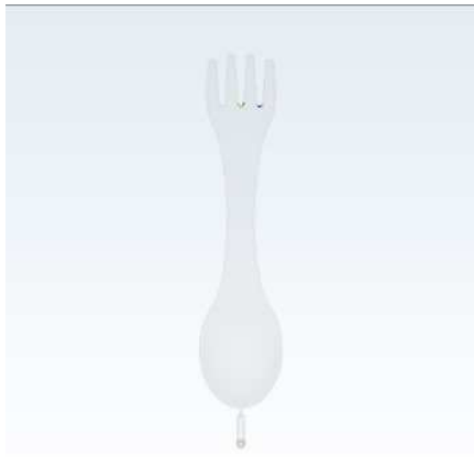
Gambar 4. Cacat weld line lokasi gate 1
