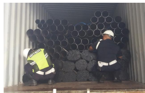
Gambar 1. Perhitungan Pipa Manual
