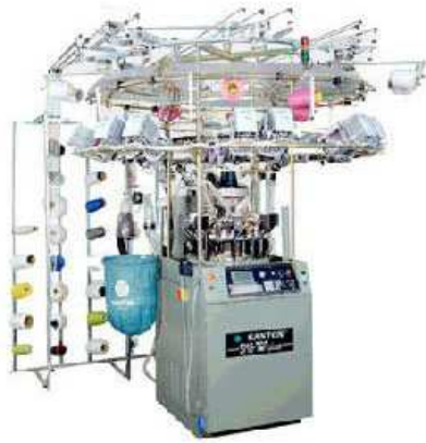
Gambar 4. Mesin Rajut Bundar Seamless - Jacquard
