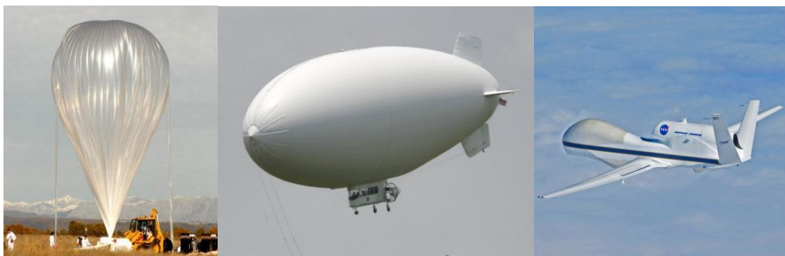
Gambar 2. Infrastruktur HAP (kiri-kanan): Balon, Airship, Aeroplane
