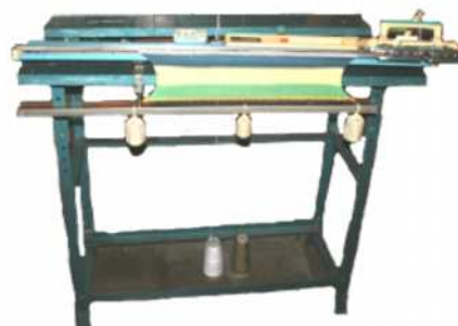
Gambar 3. Mesin Rajut Datar Single Bed Gauge 6
