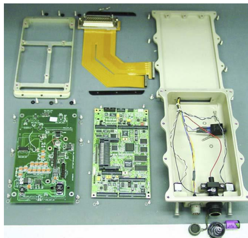
Рис. 10. Елементи Enhanced Portable Inductive Artillery Fuze Setter (EPIAFS)
