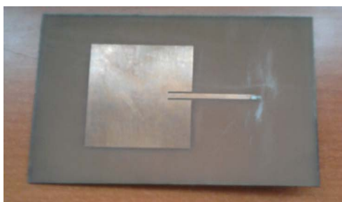
Figure 13. Fabricated Rectangular Microstrip Patch Antenna on PCB
