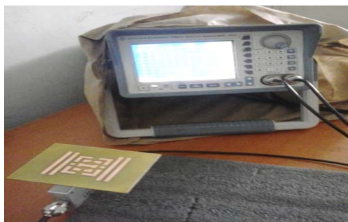
Figure 15. Setup for Measurement of Antenna Parameters
