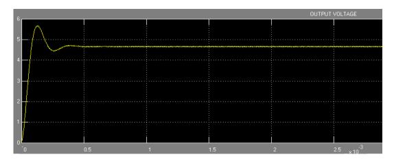
Figure 11. Output Voltage waveform of buck converter using Open loop model
