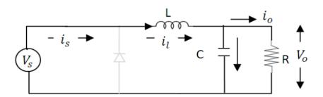
Figure 2. Equivalent Circuit during ON State
