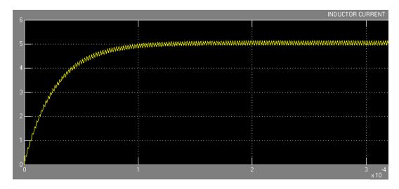
Figure 18. Waveform of Inductor Current of Buck Converter using Fuzzy Controller
