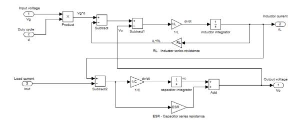
Figure 10. Subsystem of Buck Converter
