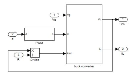
Figure 9. Subsystem of Open Loop Buck Converter
