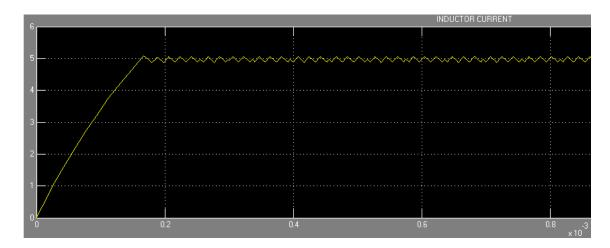
Figure 15. Inductor Current waveform of buck converter using PI Controller
