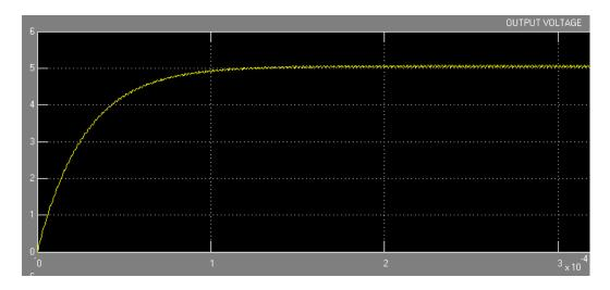
Figure 17. Waveform of Output Voltage of Buck Converter using Fuzzy Controller
