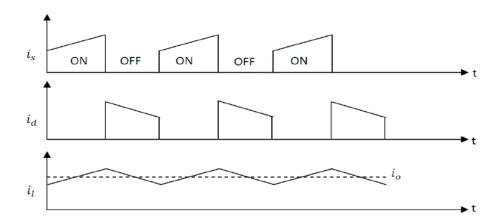
Figure 4. Waveforms of Buck Converter
