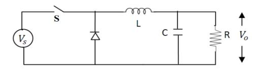
Figure 1. Circuit Diagram of Buck Converter
