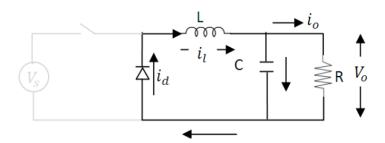
Figure 3. Equivalent Circuit during OFF State
