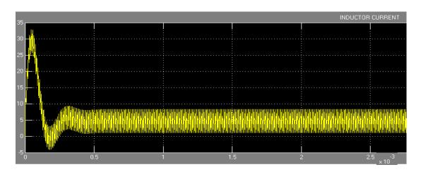
Figure 12. Inductor Current waveform of buck converter using Open Loop model
