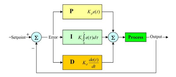
Figure 5. Block Diagram of a PID Controller
