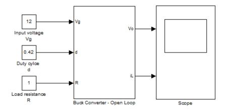
Figure 8. Simulink Model of Open Loop Buck Converter
