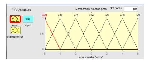
Figure 7. Membership functions for error normalized input
