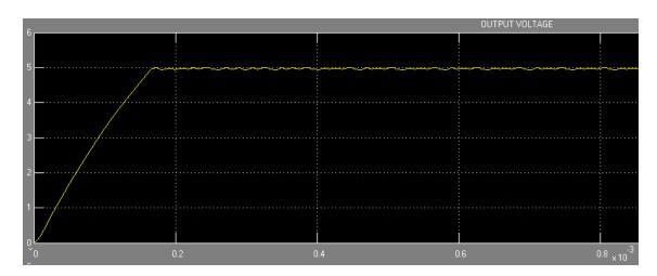
Figure 14. Output Voltage waveform of buck converter using PI Controller
