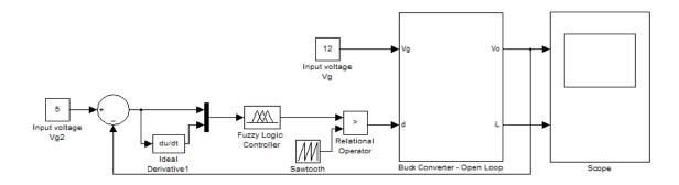
Figure 16. Simulink Model of Buck Converter using Fuzzy Controller
