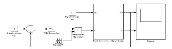
Figure 13. Closed loop model of Buck Converter using PI Conntroller.
