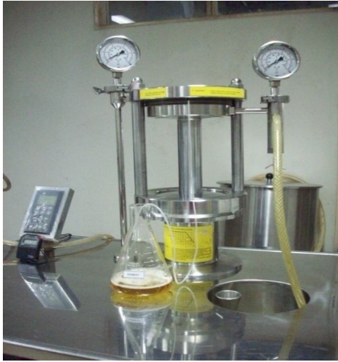
Figure 1. Cross-Flow MF/UF/NF/HF or RO module used to concentrate of LAB in mung beans vegetable broth fermented by mixed culture of Lactobacillus sp. and S. thermophilus (DSS, 2000).
