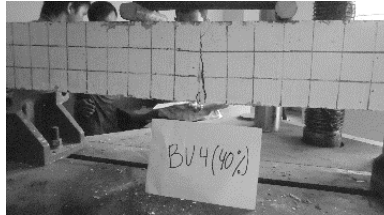
WTR-40 (Waste tire reinforced concrete with 40% tension)
