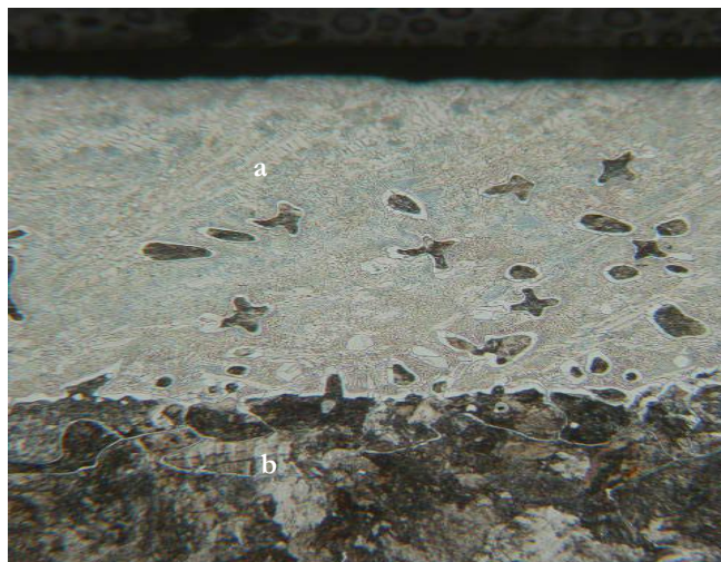
Figure 1. Optical images of borided S45C iron at 1000°C heat treatment for 8 h showing two distinct regions (a) refers to a layer having borides, and (b) refers to a substrate.
