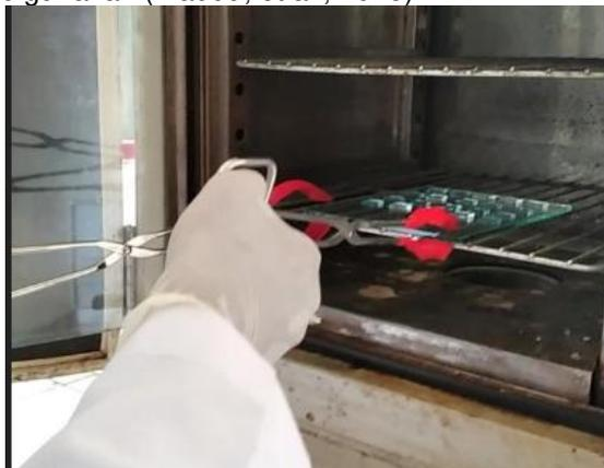
**Gambar 3.** Proses Pemanasan Sampel Lapisan Tipis  $\text{TiO}_2:(\text{F}+\text{In})$
