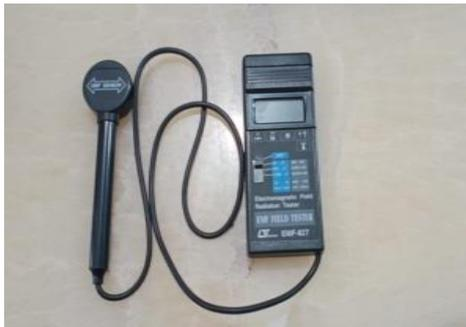
Gambar 2. EMF tester tipe Lutron EMF-827
