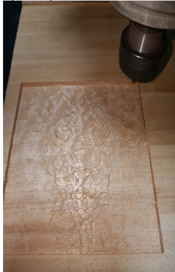
Gambar 10. Proses CNC Rough Cutting
