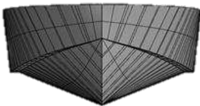
Figure 1. Body Plan of Ship
