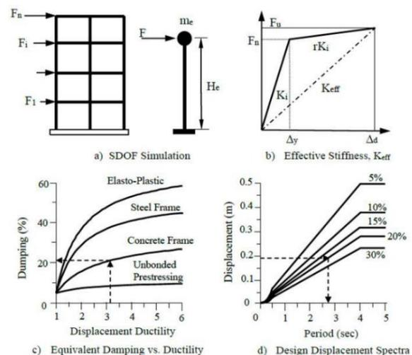
Figure 1. Direct Displacement Based Design Concept [27]
