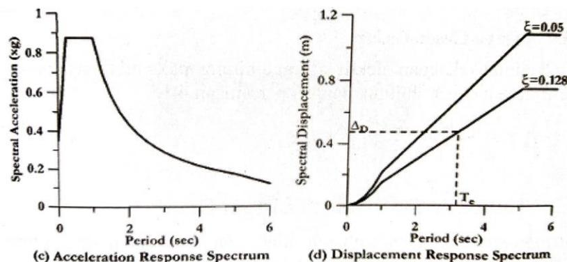
Figure 5. Response Spectrum Design and Spectra Displacement [23]
