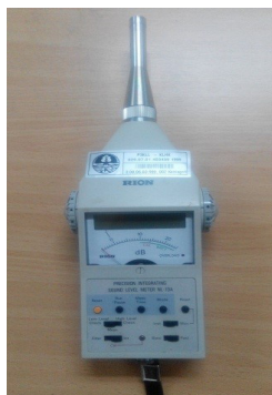
Gambar 1. Artefak SLM Rion-NL 10A
