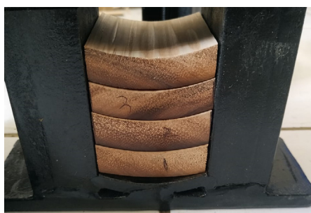
Figure 2. Laminated bamboo moulding for steam treatment
