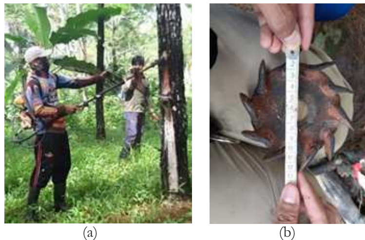
Figure 3. Tapping a pine tree: (a) hand-held tapping machine, (b) the head cutter's shape
