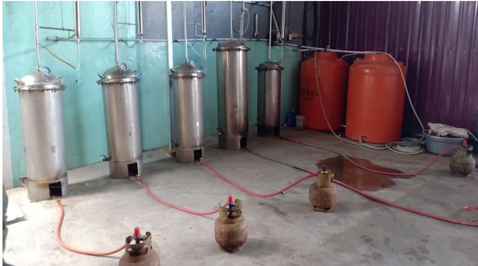
Gambar 2. Alat penyulingan minyak gaharu Figure 2. Agarwood oil refining tools
