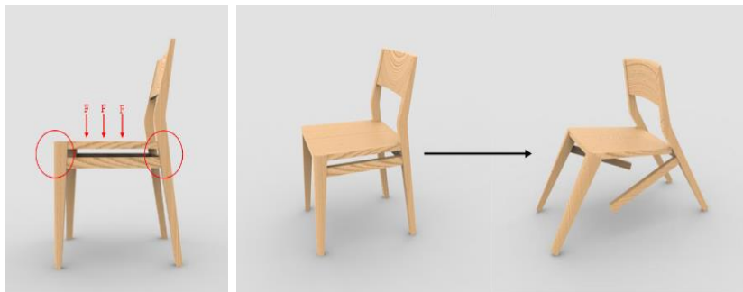
Gambar 7. Analisis kerusakan pada sistem sambungan mebel kayu Figure 7. Analysis of damage to the wooden furniture joining system
