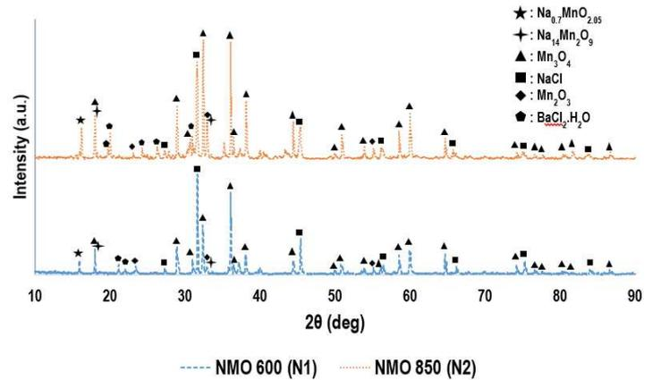
**Figure 3.** Diffraction Pattern of Samples N1 and N2
