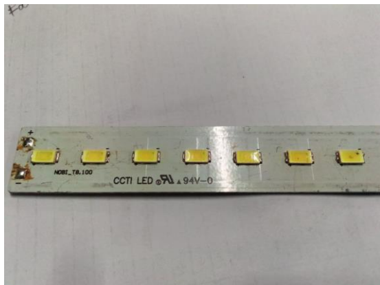
Gambar 3. LED SMD Osram Duris E3 (3.0x1.4mm).
