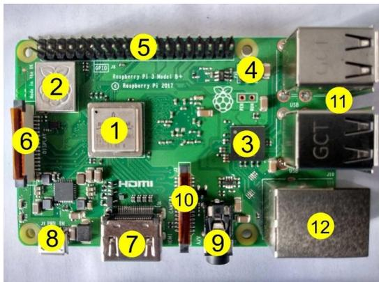
Gambar 4. Raspberry Pi 3 model B
