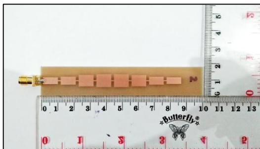
Gambar 7. Hasil fabrikasi antena fed series 1x8.
