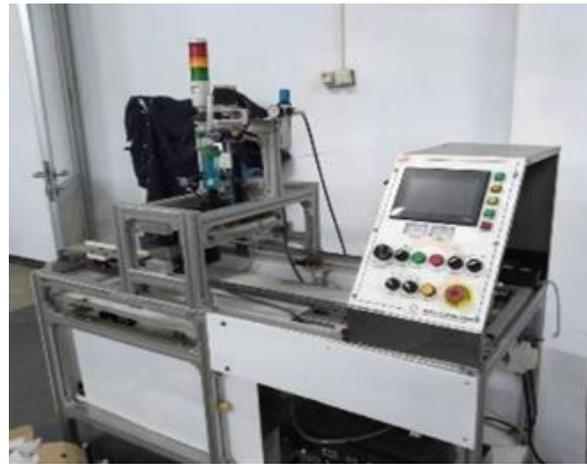
Gambar 1. Mesin plasma lucutan korona
