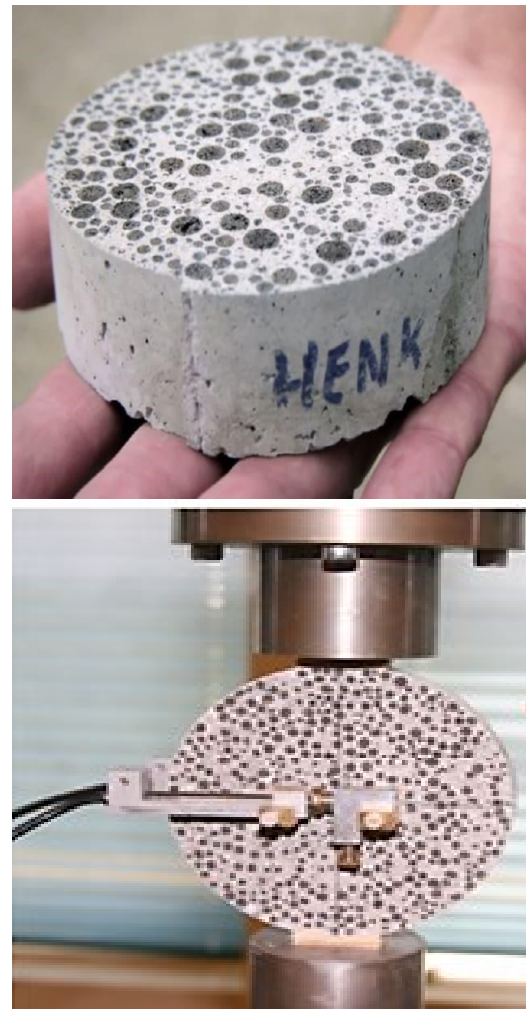
Figure 3. Bio-engineered concrete developed by the encapsulation method (Jonkers, 2011)
