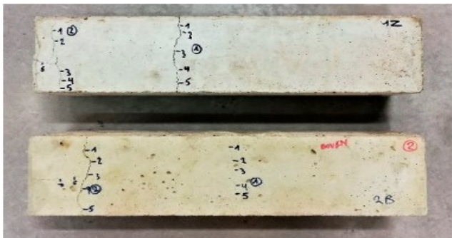
Figure 16. Laboratory prism specimens made by bio-engineered concrete (Mulleem et al. , 2020).
