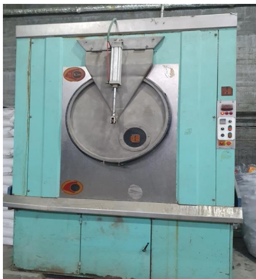
Figure 2. Tumbler garment dyeing machine, Model: K075M300
