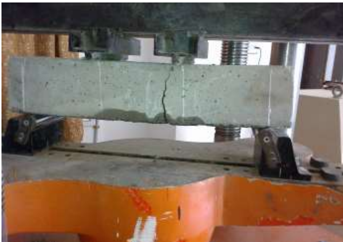
Fig. 1 - Flexural Test Setup
