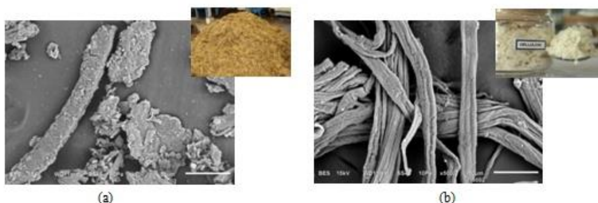
Figure 1. Results of morphological analysis with SEM (a) OPEFB; (b) cellulose
