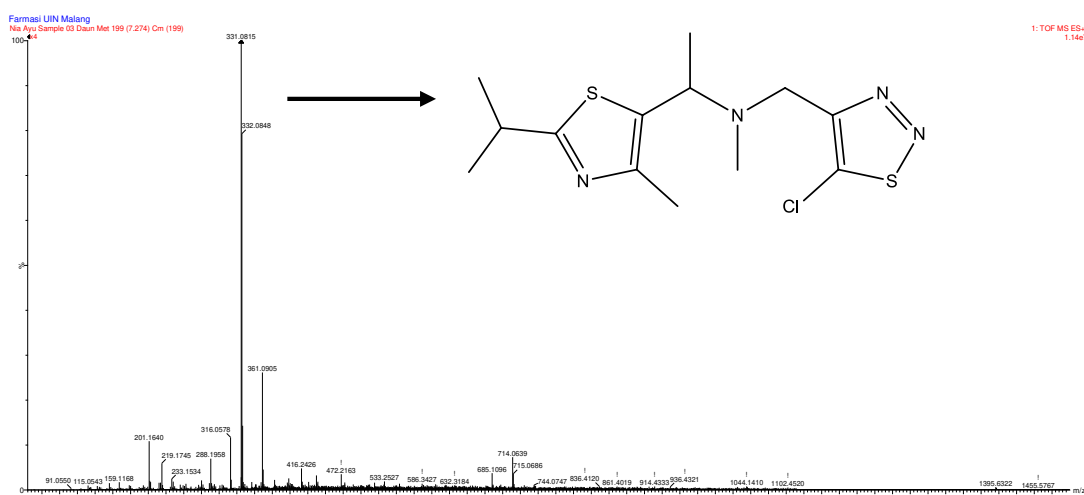
Figure 5. Spectra m/z and structure of N-[(5-Chloro-1,2,3-thiadiazol-4-yl)methyl]-1-(2-isopropyl-4-methyl-1,3-thiazol-5-yl)-N-methylethanamine
