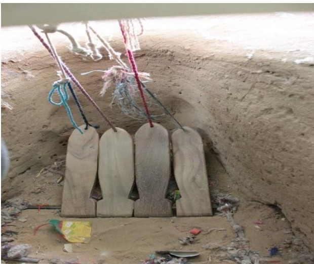
Figure 3: Treadles inside the dig to give movement to the heald shaft
