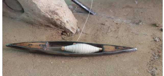
Figure 4: Shuttle carrying the weft yarn
