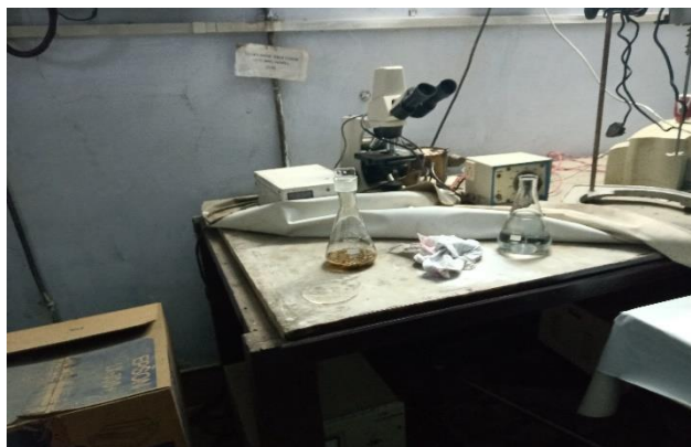
Figure 2: Lignin extracted from bagasse by alkali KOH
