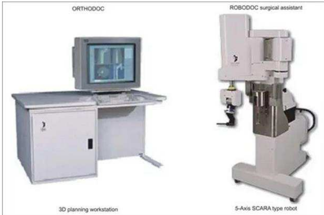
1-Figure The ROBODOC system used in surgery orthopedic
