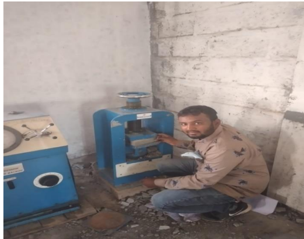
Figure 3 - Compressive strength testing on CTM
