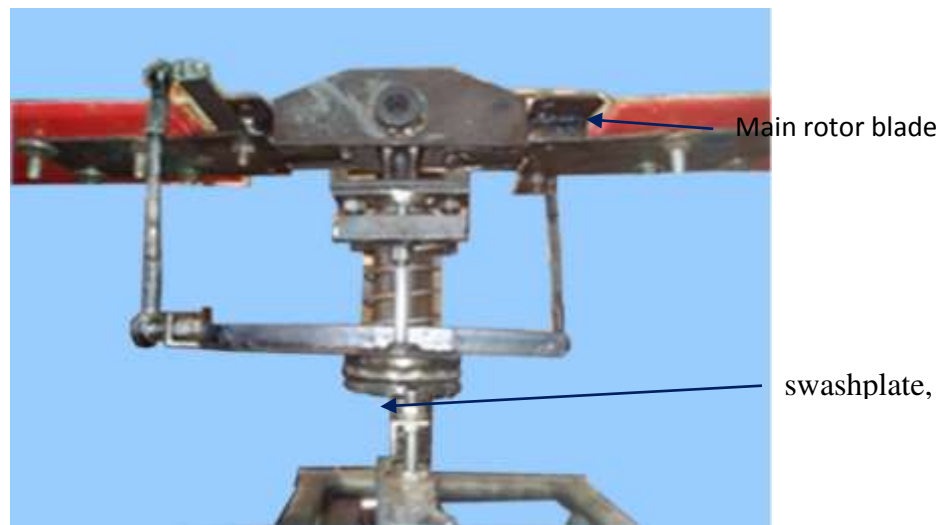
Figure 3: Construction and installation of the swashplate.
