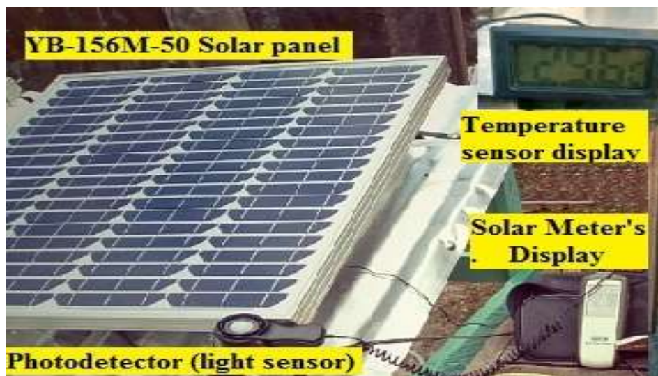
Figure 6: Experimental Setup for Data Collection
