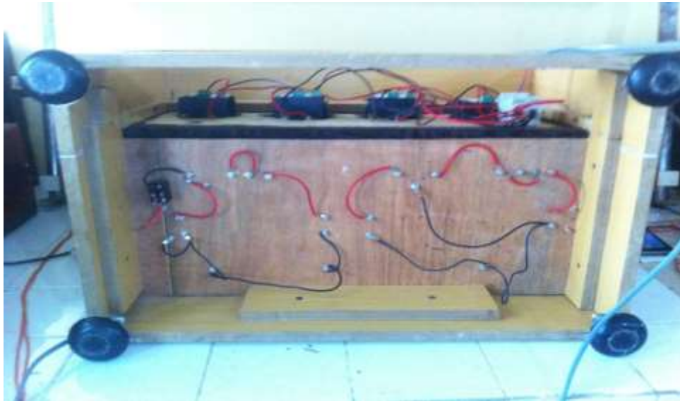
Figure6: Transformer circuit board internal connection
