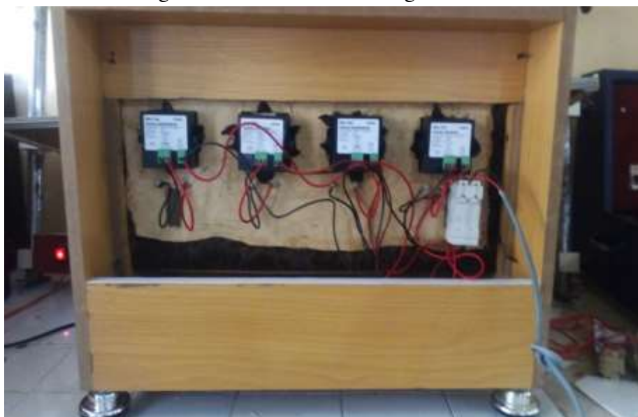
Figure5: Panel meters internal connection
