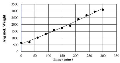
The graph depicts the relation between Average molecular weight of adduct and the time of reaction. As time increases the polymerization continues and dense mass is obtained of novel resin.
