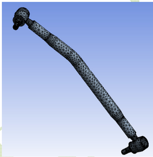
Fig.6 Meshing of three dimensional model
